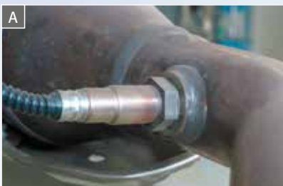
A High operating temperatures and aggressive exhaust gas place high demands on lambda sensors B Different plugs, one cable length: this reduces storage space
